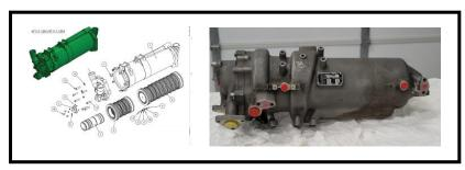
Using state-of-the-art-equipment and technology, the fuel heater receives a full array of cleaning and testing to determine leakage/damage or deformation for proper functionality. The ETP Thermal Dynamics Repair Specification allows us to Repair Cracks, Surface Corrosion, Damaged Flanges/Brackets/Ducts and Core Repair or **NuCORE** Replacement
