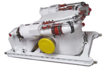
Water Separator B737
